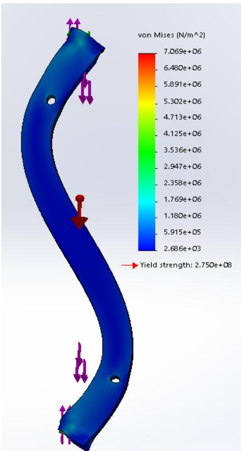
Figure 6: FEA on a fin slot where drag and thrust are applied with a large safety factor
