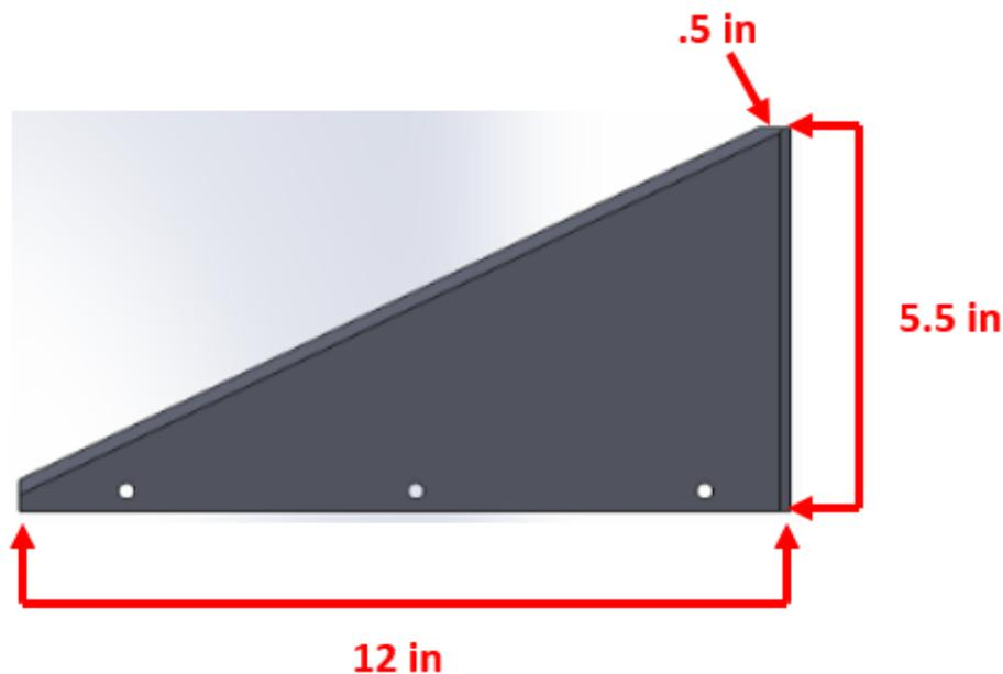
Figure 8: Front View of Fin With Dimensions
