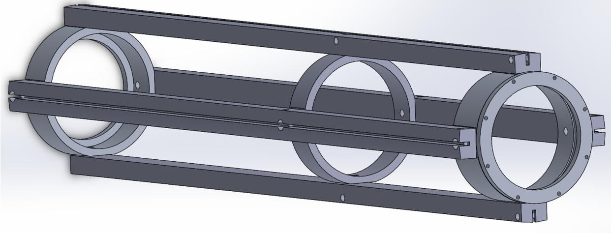
Figure 4: Motor Mount Assembly
