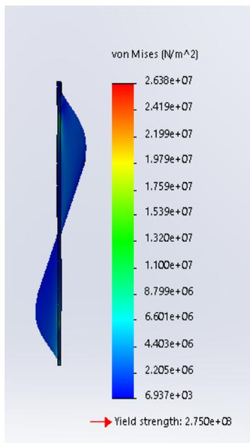
Figure 14: Max Stress from Drag Forces on a Fin
