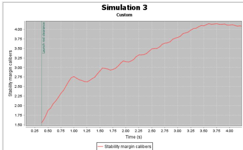
Figure 11: Stability Calibers Minimum and Maximum (Openrocket)
