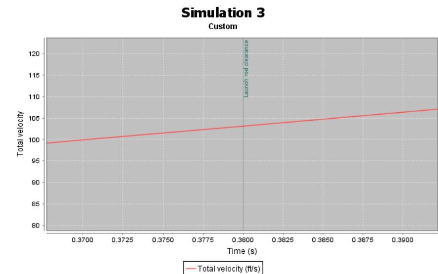
Figure 10: Velocity at Launch Rod Clearance (Openrocket)
