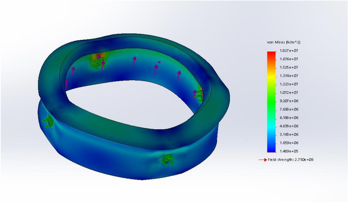
Figure 5: FEA on the upper thrust bearing cap with a safety factor of 15
